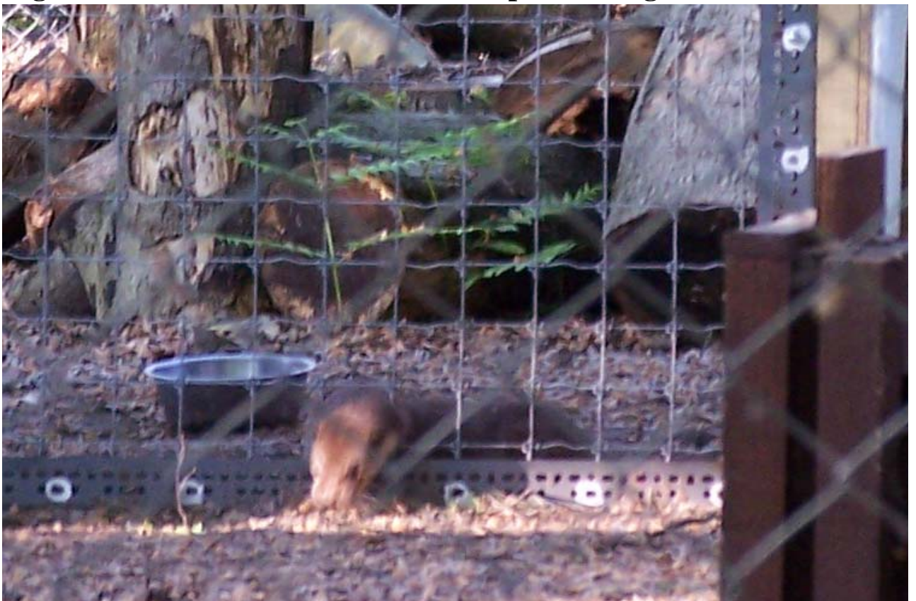
Figure 2. Small female otter unable to pass through 75mm Titan mesh
